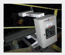
MoistScan® MA-500HD installed on the plant feed conveyor belt at a nickel ore refinery. Data from the MoistScan® is used to control the residence time of the ore in a rotary dryer.
