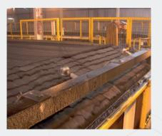
MoistScan® MA-600 installed on a horizontal belt filter at a coal wash plant. The MA-600 has 3 sets of antennae across the belt. The analyser calculates average moisture across the belt which is used to control belt speed and flocculant addition.
