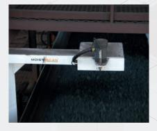
MoistScan® MA-500HDi measuring moisture content of iron ore pellets at a shipping port. The analyser is used to calculate the total dry tonnage as the product is loaded onto the ship.
