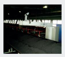
MoistScan® MA-500 installed on the coal receival belt of a power plant. The MA-500 is used in conjunction with an online elemental analyser to determine the total dry ash percentage and sulphur content of the received coal.
